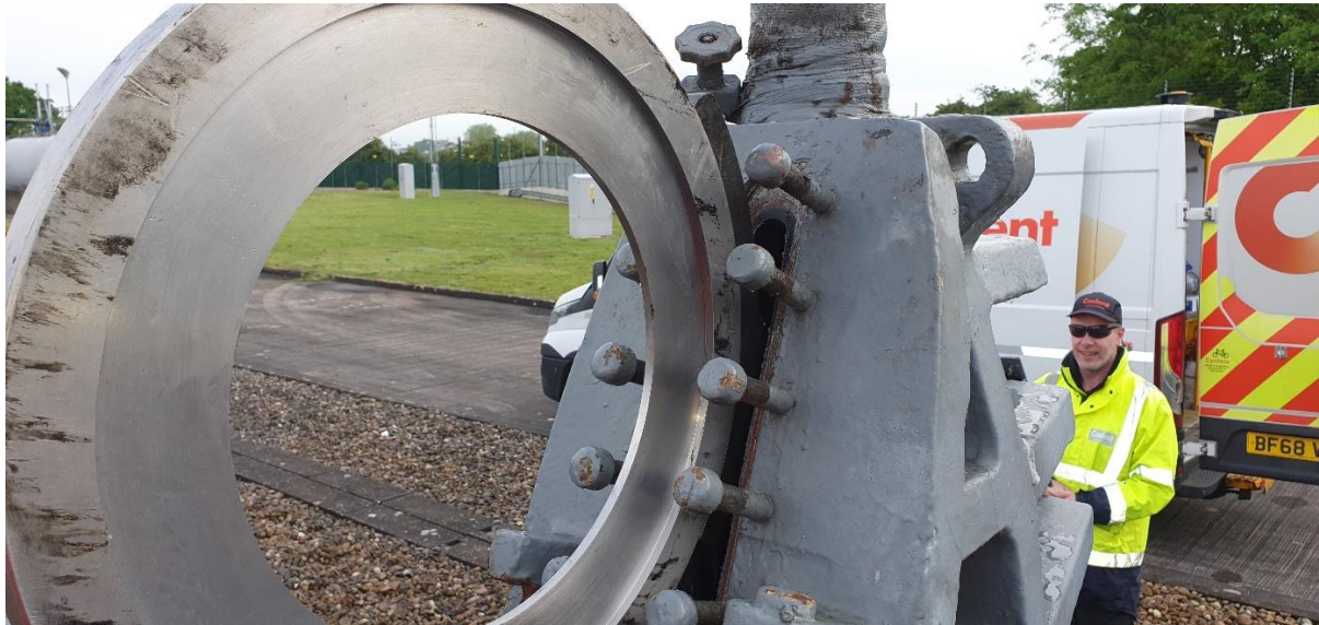
Figure 17: Flow Test 4 - Plate 2 (ARLE5036) - Sharp Edge Downstream
