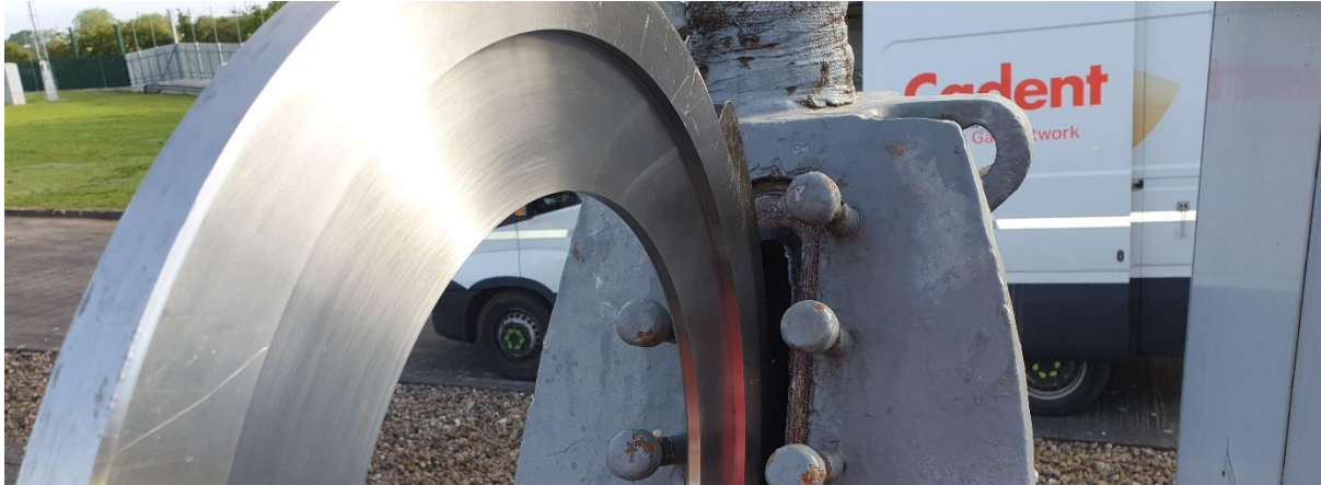
Figure 10: Flow Test 2 - Plate 1 (295/5) - Sharp Edge Downstream
