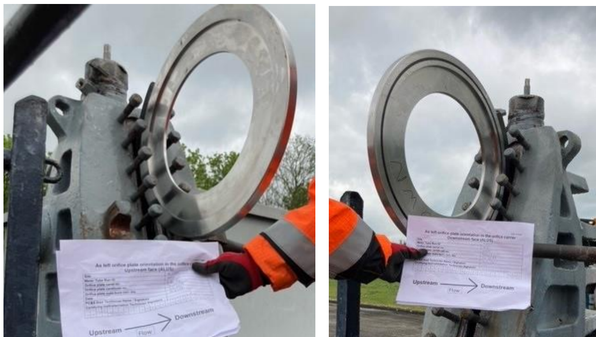
Figure 7: Flow Test 1 - Installation of plate 1 (295/5)
