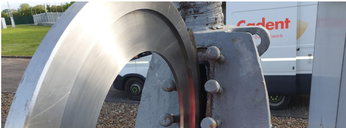
Figure 8: Flow Test 2 - Plate 1 (295/5) - Sharp Edge Downstream
