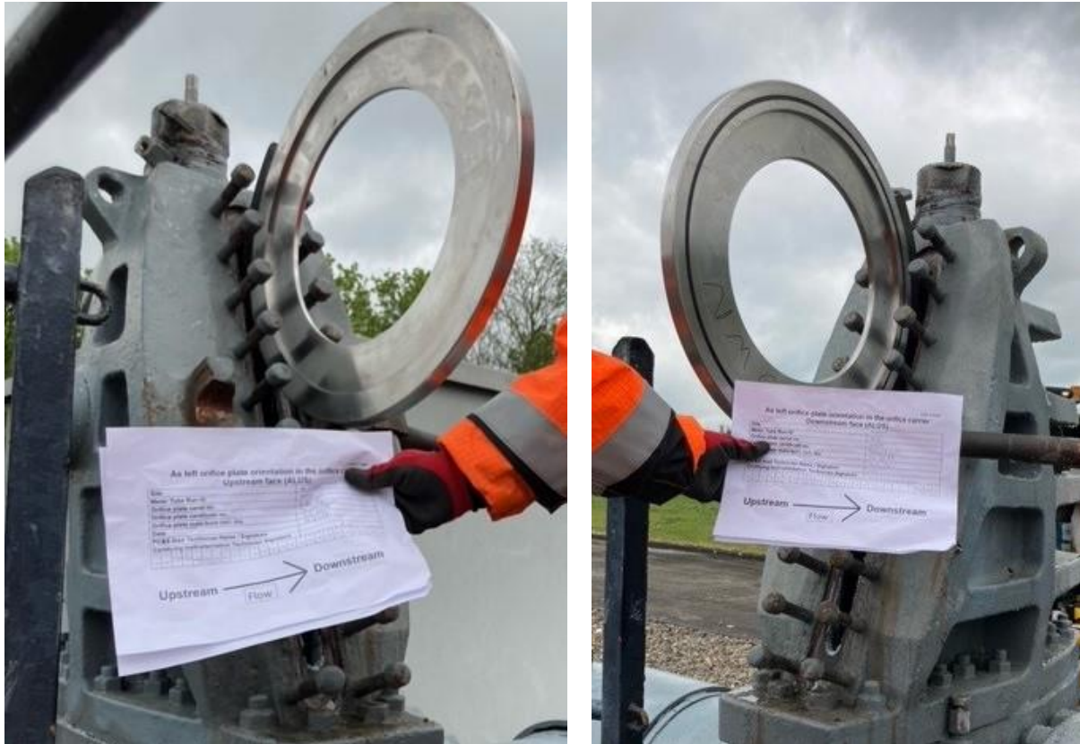
Figure 4: Flow Test 1 - Installation of plate 1 (295/5)
