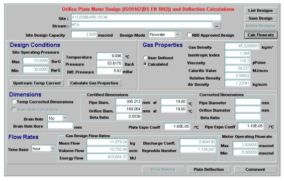
Fig. 1b - HPMIS screen shot for flow calculation using calculated average pressure value (23:12).
