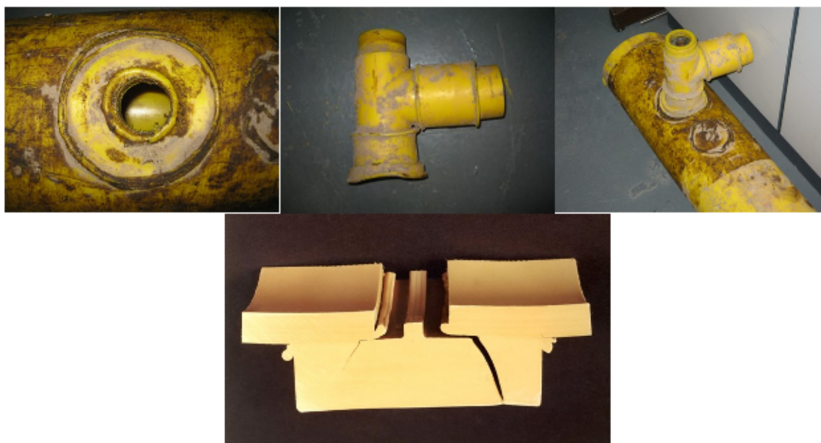
Figure 6: Examples of hot iron joint failures: saddle (upper), pipe joint (lower)
