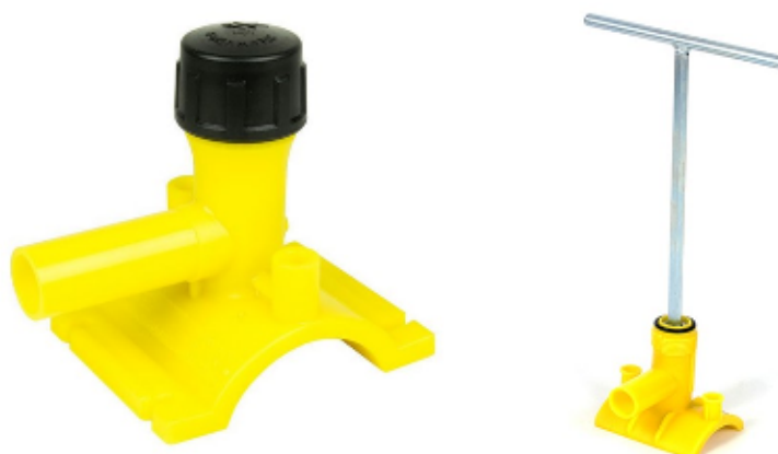
Figure 4: Electrofusion saddle tee with black completion cap (left); cap removed to operate the integral cutter, exposing elastomer seal (right)
