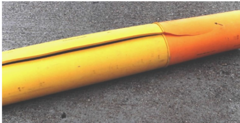
Figure 3: Improvement in RCP resistance from early PE (on left) to PE100 (on right)
