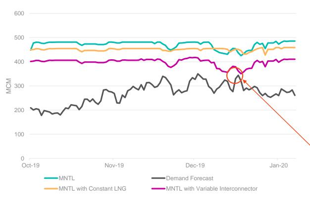
A notice that forecast demand had breached 95% of the MNTL would have triggered on 17/12/19 if the interconnector methodology had been introduced as well as the new LNG methodology
