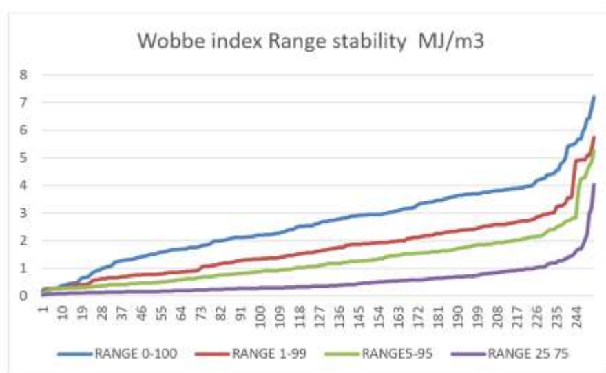
Figure 2 — Wobbe Index bandwidth for different percentiles at the 253 exit points over 2015-2016 from survey 2, analysed by JRC
