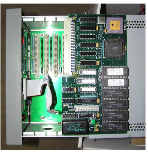
Omni 6000 Flow Computer CPU (EPROM-type) Back-up Battery and EPROM Location plus OmniCom Start-up Screen
