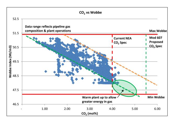
Processing commingled pipeline gas with higher CO<sub>2</sub> content may require more energy in export gas to meet lower Wobbe specification (warmer plant) depending on overall gas composition
