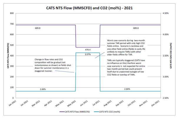
From 2019 onwards,  $CO_2$  levels in CATS/TGPP export gas during the summer months are likely to range between 2.66 mol% and 4.0 mol% with  $CO_2$  levels in non-summer months ranging between 2.66 mol% and 3.57 mol%. A representative example of the gas flow from the CATS plant and the associated  $CO_2$  content of the gas for 2021 is shown in the chart above. This is based on the high CATS pipeline flow rate (all fields producing) scenario that BP has previously shared with the Workgroup.
