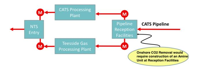
Gas in dense phase is carried from offshore oil and gas fields to Teesside by the CATS Pipeline. The reception facilities contain flow & pressure control equipment, metering and H2S & Hg guard beds. Gas is then processed in either the CATS terminal of Teesside Gas Processing Plant. Water and NGL is removed and NTS specification gas exported via metering equipment to the NTS entry points
