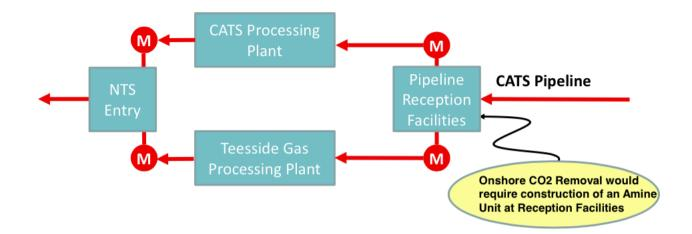
Gas in dense phase is carried from offshore oil and gas fields to Teesside by the CATS Pipeline. The reception facilities contain flow & pressure control equipment, metering and H2S & Hg guard beds. Gas is then processed in either the CATS terminal of Teesside Gas Processing Plant. Water and NGL is removed and NTS specification gas exported via metering equipment to the NTS entry points
