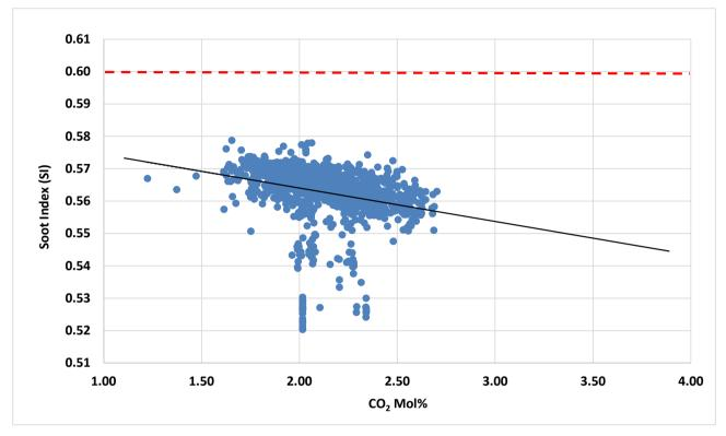
Moving from a CO<sub>2</sub> content of 2.9 mol% to 4 mol % results in a 0.01 reduction in SI.
