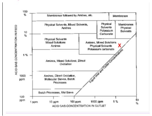
Molecular sieve technology is typically used for removing trace contaminants from gas streams and very low outlet concentrations can be achieved. The loading of CO<sub>2</sub> on molecular sieve is relatively low, and the high feed gas CO<sub>2</sub> content in this case, will result in a physically large system with high regeneration requirements and correspondingly high capital and operating costs when compared to alternative technologies.
