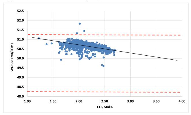
The impact on WI at 4 mol% CO<sub>2</sub> content remains well above the mid-point of the WI range allowable in the NTS gas specification. A move from CO<sub>2</sub> content of 2.9 mol% to 4 mol% would result in a decrease in WI of about 0.5 MJ/SCM.
