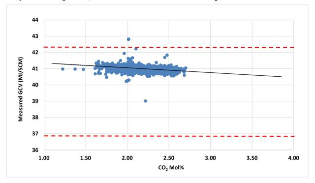
Extrapolating this to a max of 4 mol% would result in a forecast GCV of 40.4 MJ/SCM or a change of less than 1 MJ/SCM when  $CO_2$  content of the gas is 1 mol%. The analysis shows that this GCV remains significantly within the range of GCV allowable in the NEA.
