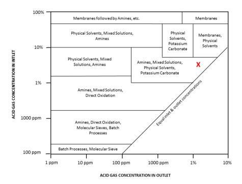
Molecular sieve technology is typically used for removing trace contaminants from gas streams and very low outlet concentrations can be achieved. The loading of  $CO_2$  on molecular sieve is relatively low, and the high feed gas  $CO_2$  content in this case, will result in a physically large system with high regeneration requirements and correspondingly high capital and operating costs when compared to alternative technologies.
