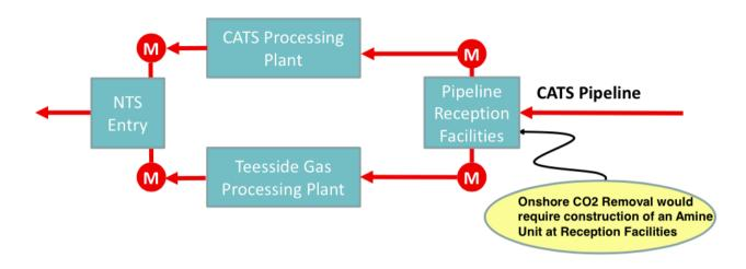
Gas in dense phase is carried from offshore oil and gas fields to Teesside by the CATS Pipeline. The reception facilities contain flow & pressure control equipment, metering and H2S & Hg guard beds. Gas is then processed in either the CATS terminal of Teesside Gas Processing Plant. Water and NGL is removed and NTS specification gas exported via metering equipment to the NTS entry points
