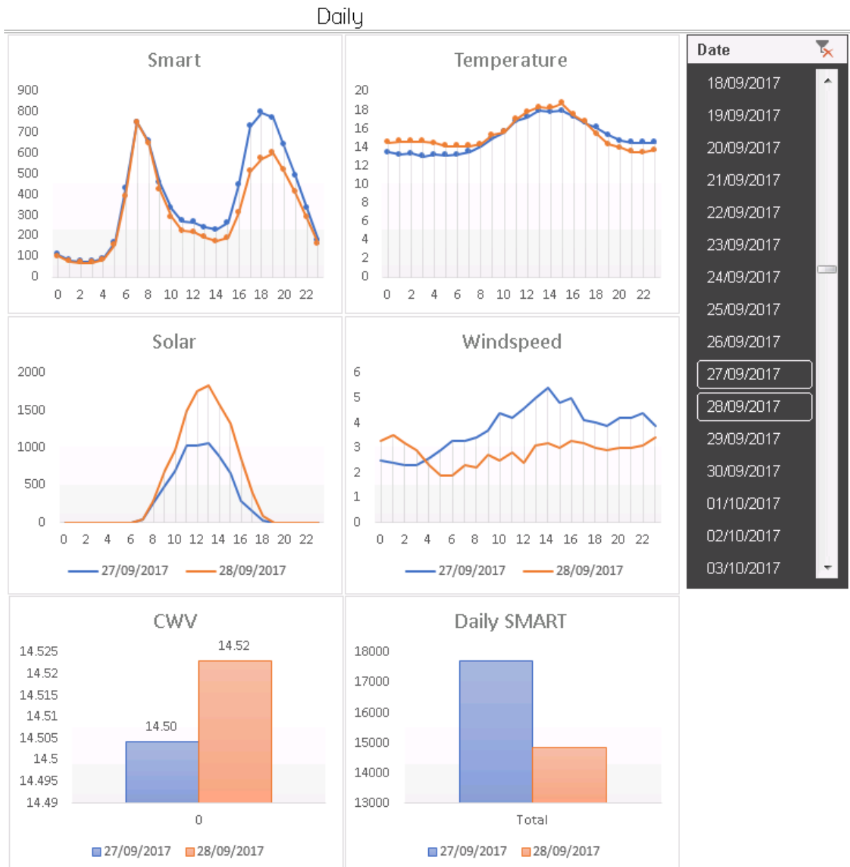
Figure 1:27/09/2017 – Wednesday. Levels of solar across the day were low, with CWV at 14.50 and 14.52 for the comparison day. Daily demand differed greatly as a result of higher evening peak demands. An explanation could be due to more heating demand needed following the low levels of solar radiance during the day. However wind speed was also higher, perhaps this could be the reason for higher peak demand. Given CWV is in the transition range it would have no effect on the CWV calculation, if it had CWV would had been lower.
