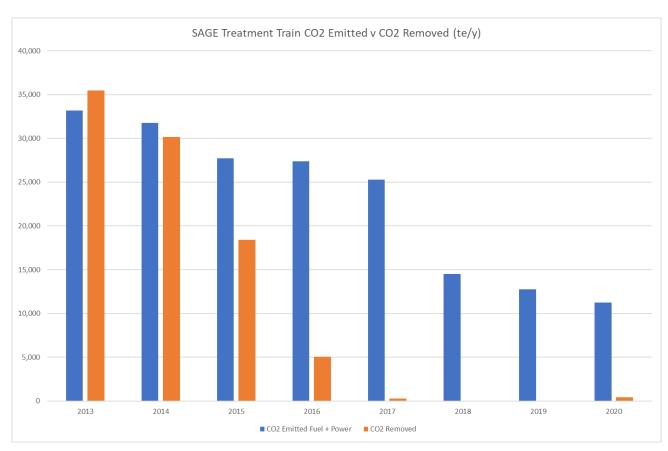
For example, in 2020 more than 12000 tonnes of  $CO_2$  were emitted to remove (and emit) 400 tonnes of  $CO_2$ . To date this year only 74 tonnes of  $CO_2$  have been removed.
