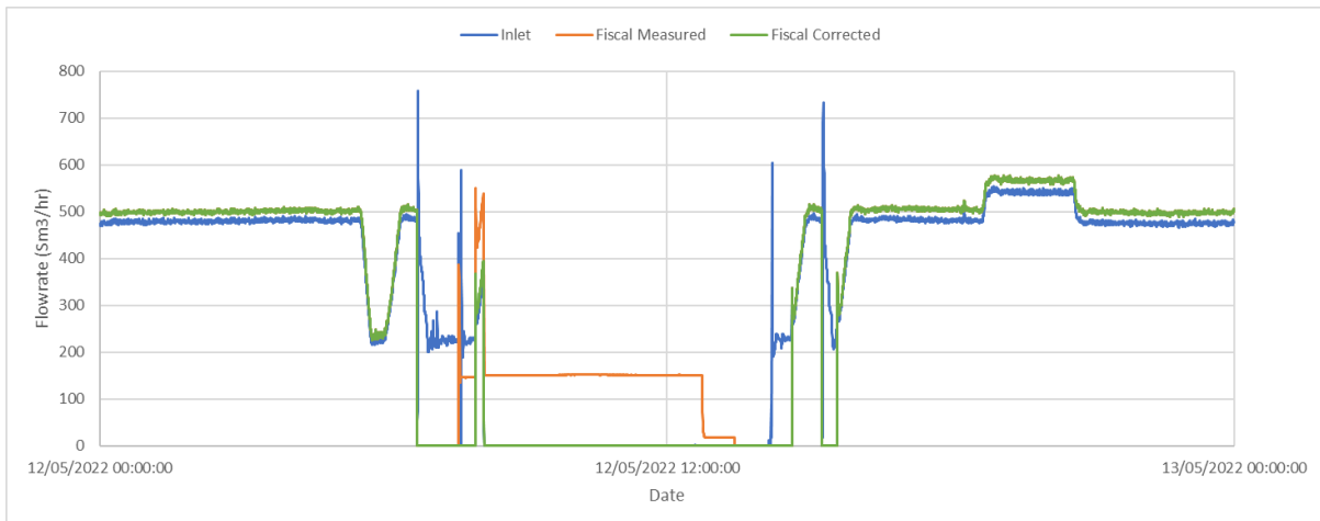
Figure 2 Volume flow rates for Fiscal USM, Inlet USM and corrected Fiscal USM (12/05/2022)
