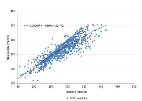
Figure 1 – Non storage supply (NSS) versus demand for the winters 2015/16 to 2018/19
